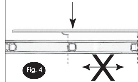
Fig. 4 shows correct alignment of lip and lugs to prevent sideways movement.
