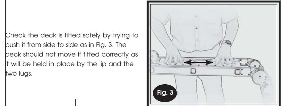
Check the deck is fitted safely by trying to push it from side to side as in Fig. 3. The deck should not move if fitted correctly as it will be held in place by the lip and the two lugs.
