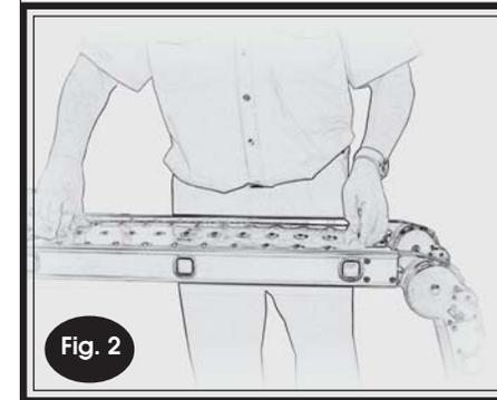
Lower the deck until it lies flat, (Fig. 2) with the lip pushed up to the first ladder rung. The other end of the deck should be covering half of the rung it is lying on.
